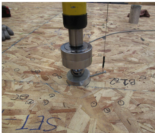
Figure 5. Close up view of puck, ball, and string to measure deflection.
