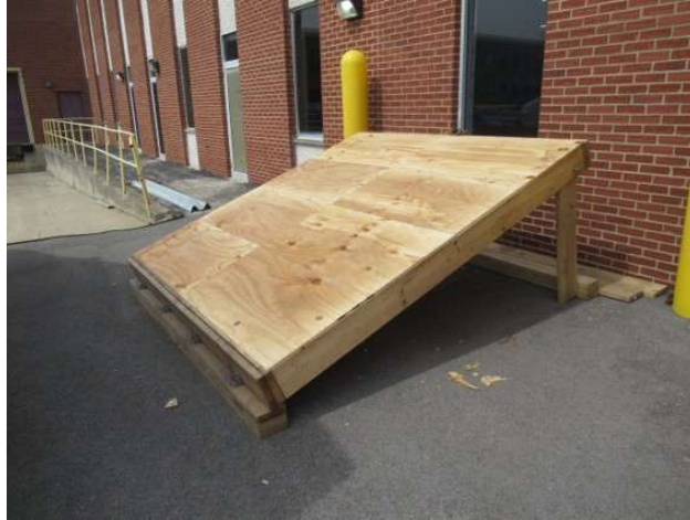
Figure 7. Test frame lifted to 4:12 pitch for exposure,
