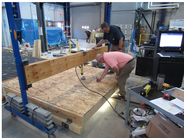
Figure 4. Concentrated load test setup.
