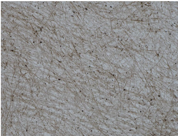
Figure 7. Fiberglass reinforcement from a modified bitumen base ply.
