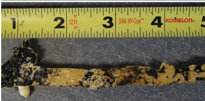
Fig.2 Close up of another field sample of hard ,glassy off ratio foam with some adhesive ability but not much for on the roof. Note in Figure 1 the foam bead is skinny, has not risen and nothing is adhering to it as the insulation boards freely buckled upward. Figure 2 shows a similar condition on a different roof; thin bead of foam, (3/8"wide) with spotty adhesion. Not good at all.
